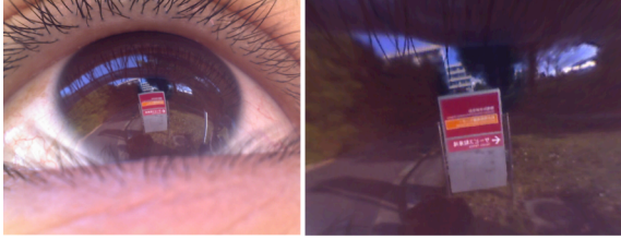
Figure 6. Result of generating unwarped corneal surface image. Left and right images are input image and generated unwarped corneal surface image respectively.
